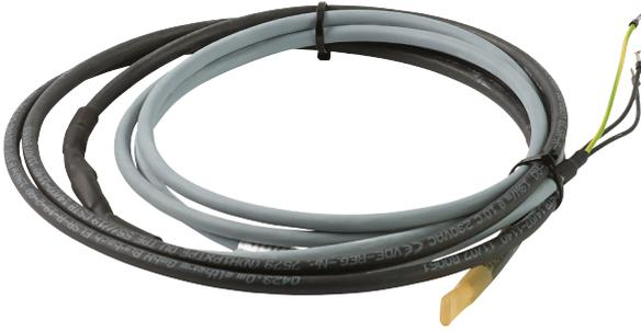
Self-limiting flexible ribbon heater to keep the condensate connection for air | water heat pumps free of ice. Both versions have a 2 m connecting cable. Heated length: HZB-1: 1 m; HZB-2: 2 m.
