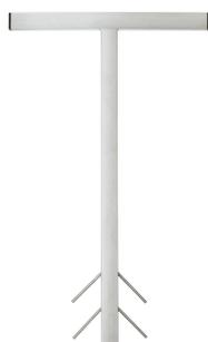
Stainless steel, T-shaped support for floorstanding, concrete-embedded installation. Standard delivery includes: 2 pce incl. installation aid for a defined clearance dimension, anti-vibration mounts, plus 1 m self-limiting ribbon heater.
