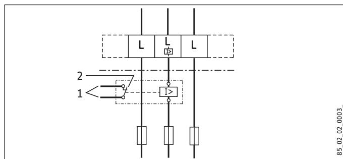
1 Control cable to the contactor of the second appliance (electric storage heater, for example).
