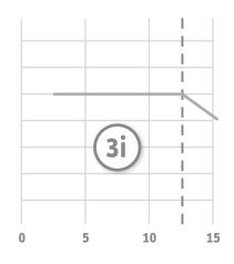
Constant DHW temperature up to the output limit, then decreasing at higher flow rates
